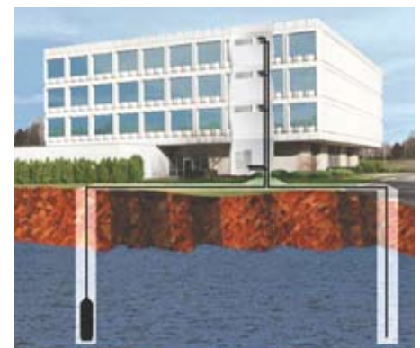
Open loop GSHC system showing abstraction and injection wells
